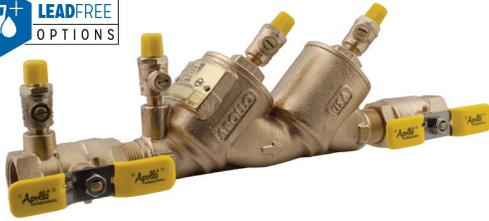
The Apollo Model DC 4A or DCLF 4A Double Check Valves are designed to prevent contamination of the potable water supply due to back-siphonage or backpressure from substances that are objectionable, but non-health hazards. The modular check valve captured spring cartridges have replaceable seats and reversible silicone seat discs. Ball valve shut-offs with stainless steel handles and nuts are standard.
