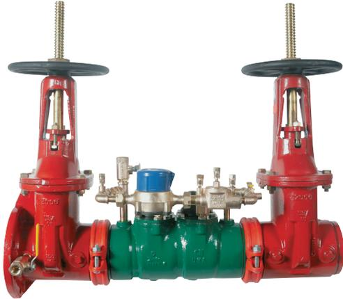
The Apollo DCDA 4SG Series Double Check Detector Assembly is designed to prevent contamination of the potable water supply due to back-siphonage or backpressure from substances that are non-health hazards. The device consists of a mainline double check valve with resilient seated shut-off valves. The bypass serves to measure water use of up to 3 gpm. Grooved connections on an epoxy-coated ductile iron body allow for easy connection to butterfly valves or gate valves. (2-1/2" - 8")
