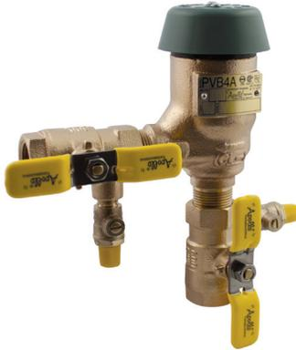
The Apollo Model PVB 4A or PVBLF 4A Pressure Vacuum Breakers are designed to prevent contamination of potable water due to back-siphonage. An integral relief valve serves to reduce the possibility of damage due to intermittent freezing conditions. The modular check valve cartridge has a replaceable seat and a reversible silicone seat disc. Ball valves with stainless steel handles and nuts are standard.
