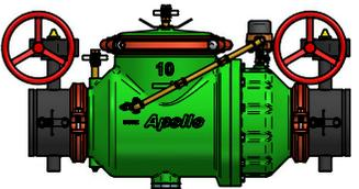
The Apollo Model DCDALF 4A / DCDA2LF 4A Double Check Detector Assembly is designed to prevent contamination of the potable water supply due to back-siphonage or backpressure from substances that are objectionable, but non-health hazards. The TriForce™ center stem guided check valves feature replaceable and reversible silicone seat discs. The bypass assembly serves to measure accurate water use of up to 2 GPM. Available in a wide variety of shut-off options.
