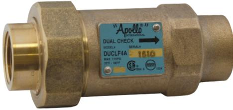
The Apollo International™ DUCLF 4A Series Dual Check Valve Backflow Preventer is designed to prevent cross-connections of non-potable water (non-hazardous) into safe drinking water systems. It is a compact and economical device that consists of two independently-acting, spring-loaded check valves in a corrosion-resistant material.
