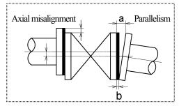
4) Tighten the bolts and nuts gradually with a torque wrench to the specified torque level in a diagonal manner. (Refer to fig.1.)
