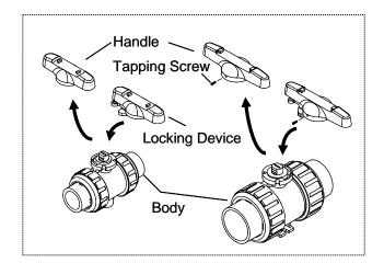
The location hole for the lock is already installed in the handle. (Table 1)
