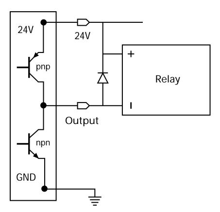
Fig. 13: Connecting Output Q1 to relay
