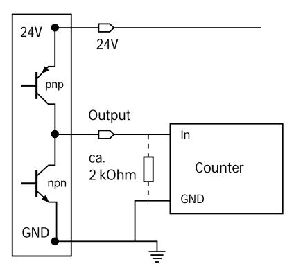
Fig. 14: Connecting output Q2 to counter
