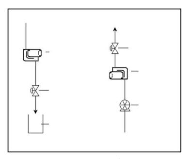
Fig. 3: Mounting examples for Flowmeter
