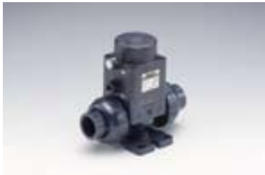
HDV12/AD16 Diaphragm Valve Socket, Threaded, Flanged 72.5 psi 15 - 25mm 58 psi 32 - 50mm
