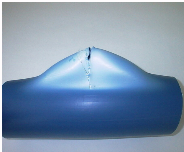
Air-Pro® over-pressurized ductile failure during burst test (pressure > 800psi)
